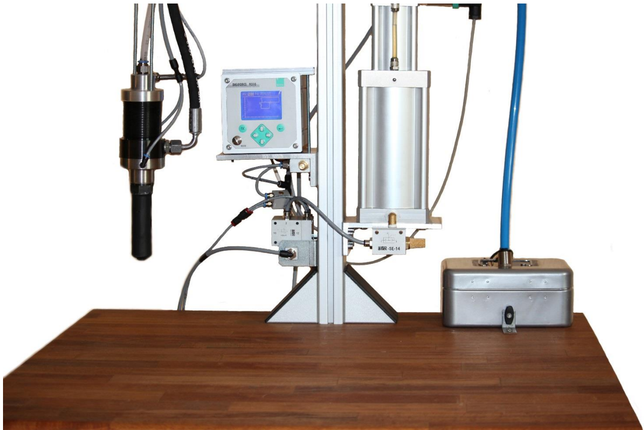
Tool for plugs, process monitoring Digiforce 9310, pressure booster and mandrel container
