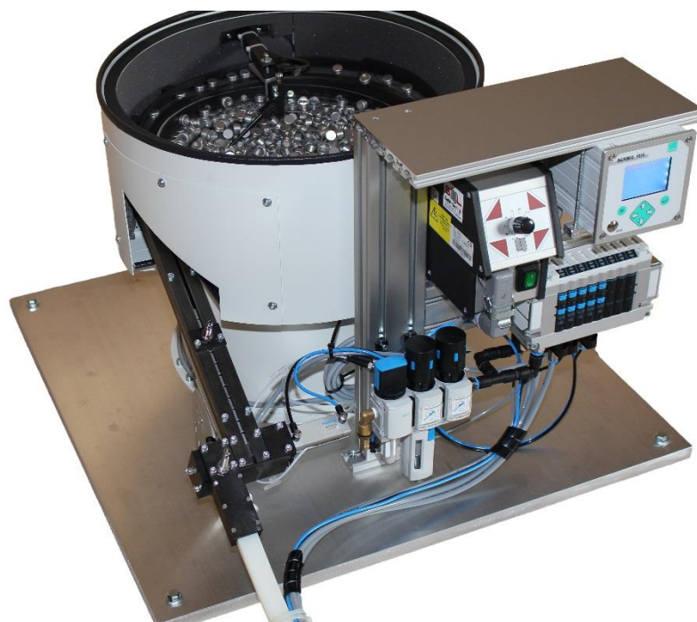
Feeding system with sound insulation and separation
